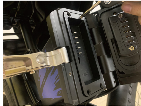
Open the controller by loosening the four screws
