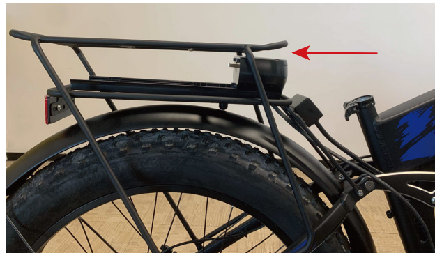
Put the base plate into the groove from the head side
