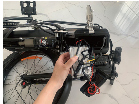
Pull all of the things out of the frame (including wires and the controller box)
