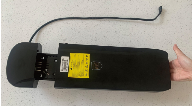
Pull out the battery from the base plate
