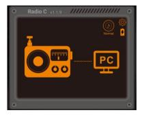
Whenever the radio is connected via USB to a PC it is possible to select PC mode. When PC mode is selected and a TF card has been inserted in the TF card slot on the right side of the radio the content of the inserted TF card is shown on the PC as a separate drive. This makes it convenient to store music files onto the TF card without having to remove it from the radio.
