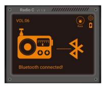
In order to use the Bluetooth audio mode, a Bluetooth capable audio streaming device needs to be connected via Bluetooth to the radio. As soon as the connection is established (message "Bluetooth connected!") you can use the normal navigation keys on your mobile device and the navigation keys [PD], [D] and [D] on the radio to control the audio playback.
