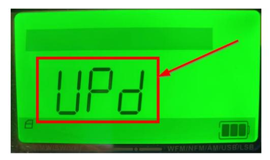
ATTENTION: Under no circumstances, remove the microSD/flash card from the RF919 or disconnect the radio from its external power supply during the update. Also do not press any keys on the radio. The update process will take a about 10 seconds.
