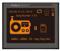
Left to the equalizer setting, the current playback mode is visualized according to the below table. Short press the symbol to change the playback mode.
