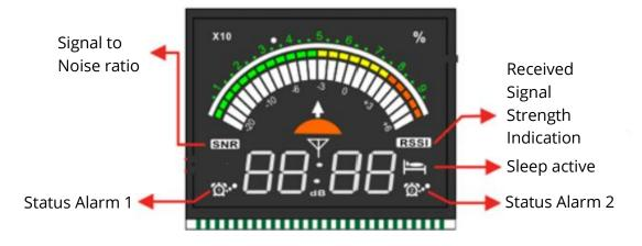
Most of the working parameters are displayed on the primary screen. However, some parameters are visualized on the secondary screen. Those are:
